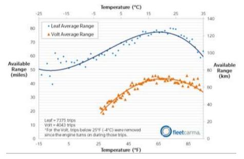
Figure 4: Range vs Temperature for Nissan Leaf (BEV) and Chevrolet Volt (PHEV) (FleetCarma, 2014)
