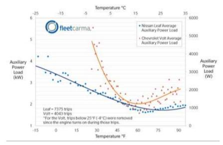
Figure 5: Average Auxiliary Power Load vs. Temperature for Nissan Leaf and Chevrolet Volt (FleetCarma, 2014)
