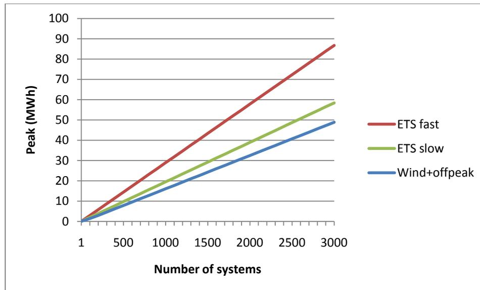
**Figure 7: The effect of different recharge algorithms on the peak in off-peak supply**
