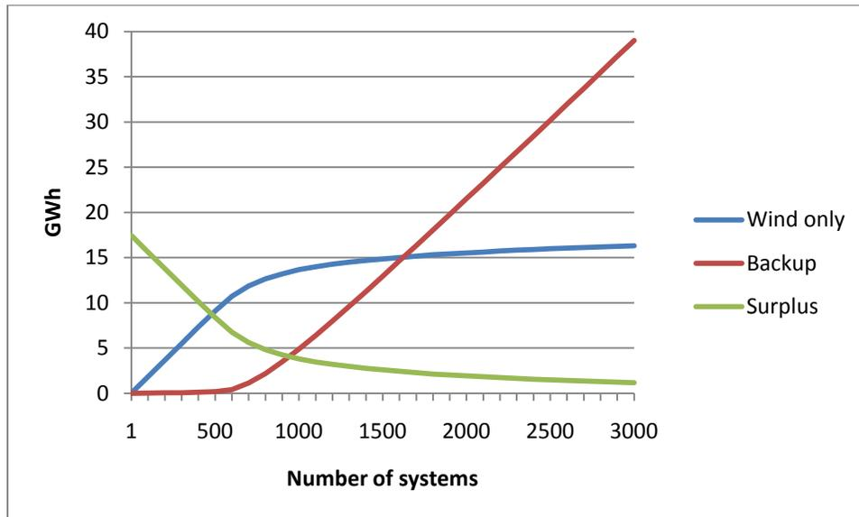
Figure 4: Increasing need for backup energy supply as the number of systems increases
