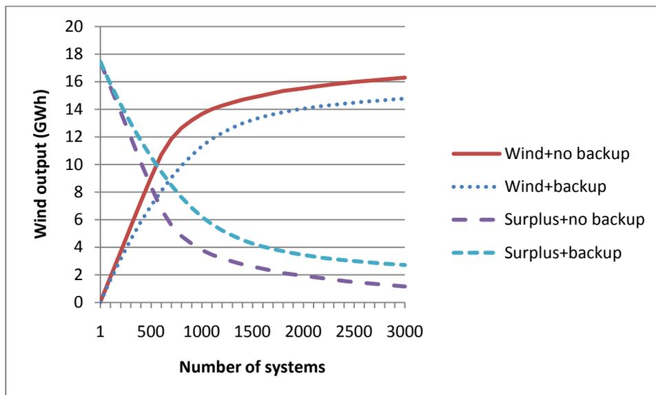
**Figure 6: Wind supply and surplus with and without off-peak grid backup.**
