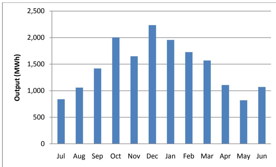
Figure 1: Monthly output from North Cape wind farm for 2002-03 heating season
