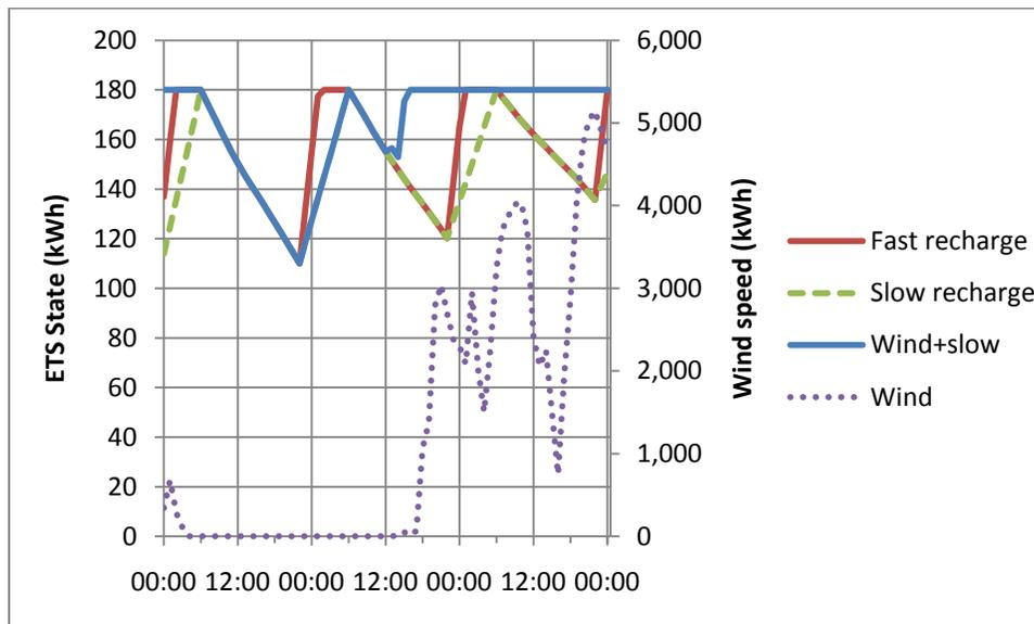
**Figure 8: The state of three different thermal storage systems over a three day period**
