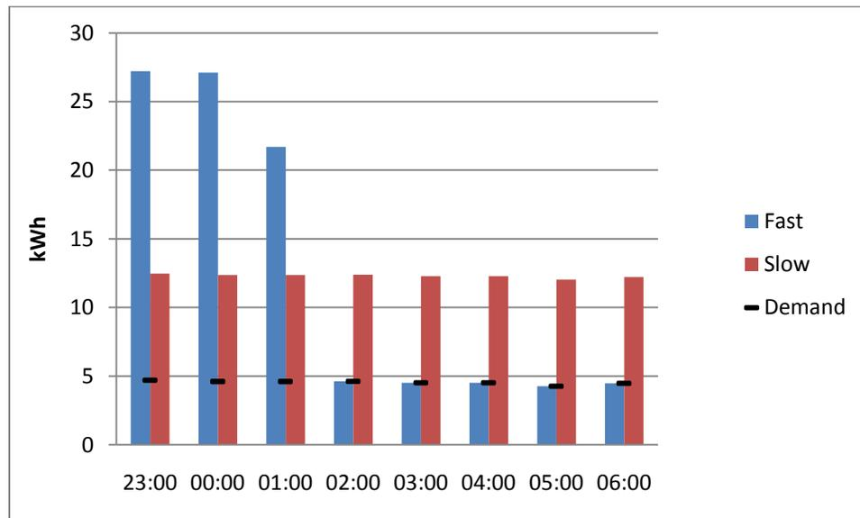
**Figure 3: Example of fast- and slow-recharge rates**
