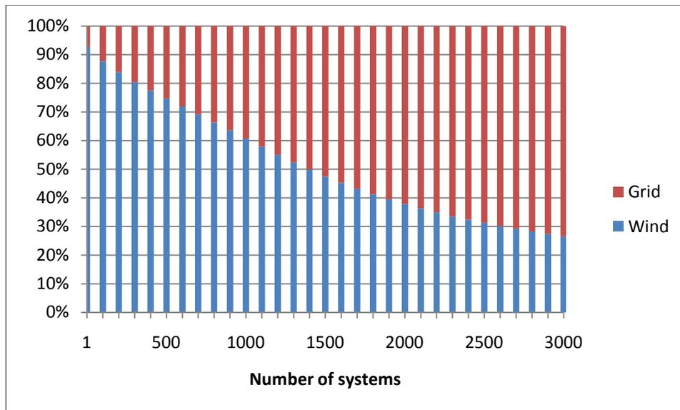
**Figure 5: Percentage of wind meeting the heating demand of thermal storage units**
