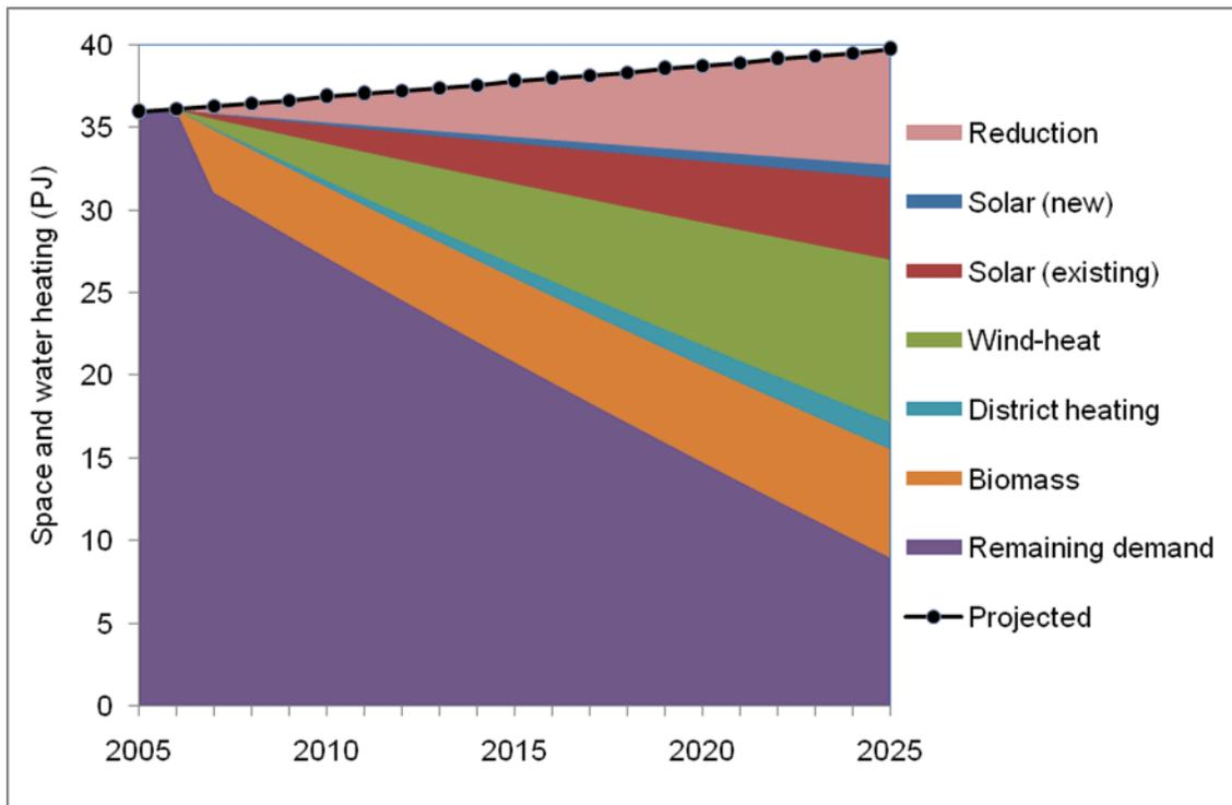
**Figure 6: Example space and water heating replacement wedges**
