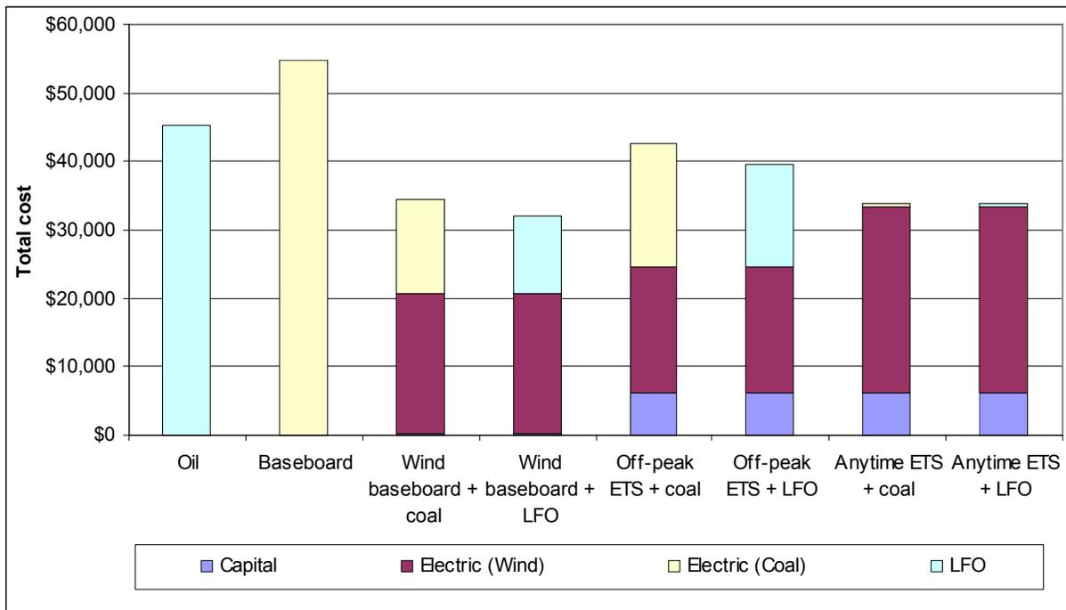
**Figure 10: Net present value of the different heating systems**
